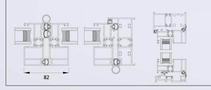
SF63 BI-FOLDING DOOR (SCHEME 633) WITH LOW BOTTOM RAIL WITH THERMAL BREAK PROFILES
