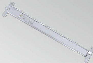
GY-SSC15 Restrictor brace (heavy duty - profile thickness 1.5mm)
